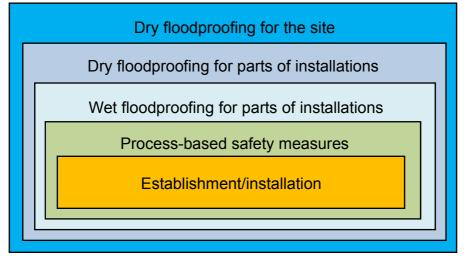
Figure 4: Safety precautions and measures (flooding)
