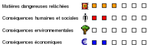
Figure 6.7 European gravity scale of industrial accidents as used by the ARIA database
