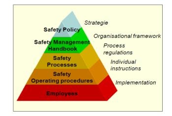
Figure 1: Hierarchy of an SMS
