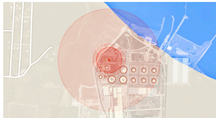
Figure 6: RAPID-N output for release of a flammable substance from a storage tank upon earthquake impact.
